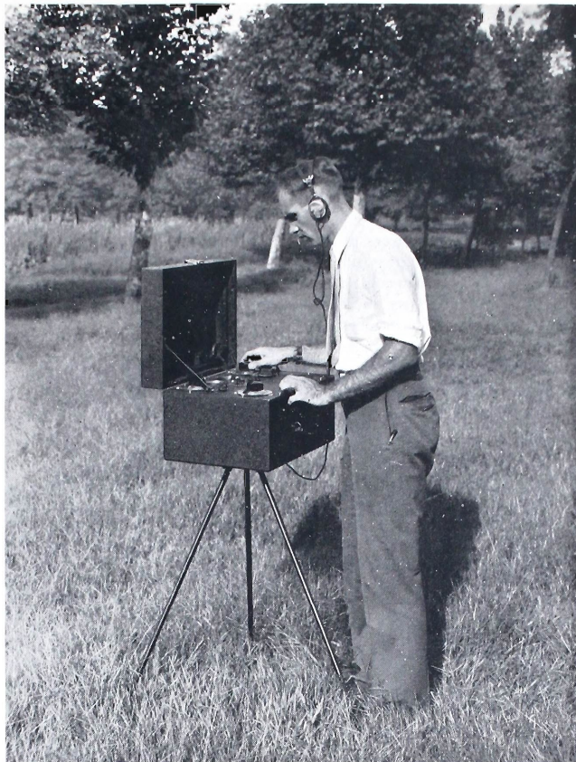
FIG. 4. NEW TYPE TMJ-21 FIELD INTENSITY METER BEING USED IN THE FIELD BY MR. GIHRING, RCA VICTOR ENGINEER. NOTE COMPACTNESS AND CONVENIENT TRIPOD MOUNTING.
